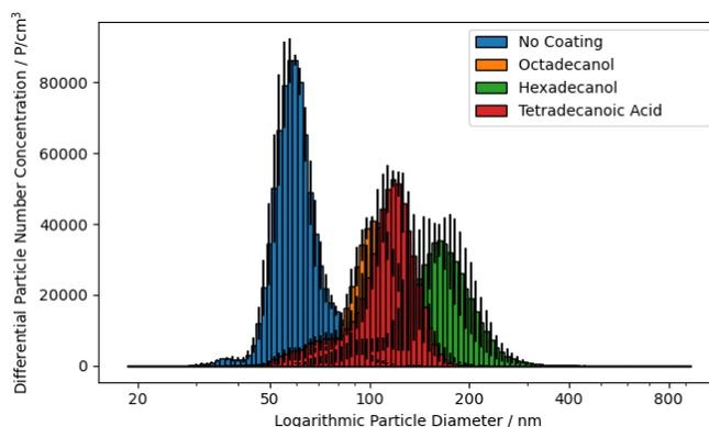
Differential Particle Number Concentration over the Logarithmic Particle Diameter of Spark-Discharge-Generated Soot, Coated with Different Substances.
