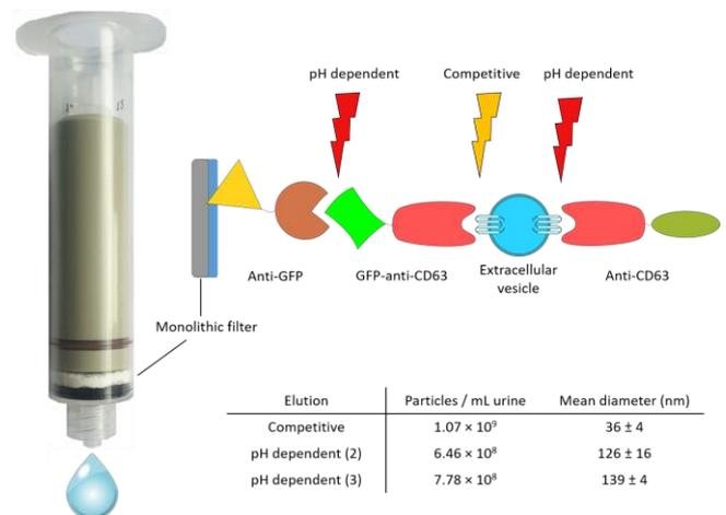
Filtration module for monolithic immuno-filtration with schematic illustration of capture and elution of extracellular vesicles from monolithic filter using nanobodies. The table shows the particles found in the elution fractions for competitive (one fraction) and pH dependent elution (2 fractions).
