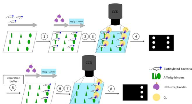
Concept of the screening assay. (1): Capture of the biotinylated bacteria through the affinity binders depending on the affinity. (2): Binding of the HRP-labelled streptavidin. (3): CL reaction. (4): Image acquisition. (5): Desorption of bacteria by desorption buffer depending on reversing of affinity. (6): Binding of the HRP-streptavidin. (7): CL reaction. (8): Image acquisition.
