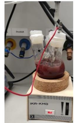
Testing *Rhodopseudomonas pentothentaxigens* for its exoelectrogenic power – Fed batch reactor with a three-electrode set-up (GE: counter electrode, RE: reference electrode, AE: working electrode, MW: medium exchange).
