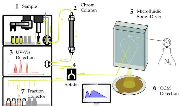
A flow splitter (4) was installed after the UV detection (3) and before a fraction collector (7). Using a split ratio of 200:1, the high flow (i.e., 99.5%) is collected (7) for later isotope analysis, whereas the low flow (i.e., 0.5%) is directed to a microfluidic spray-dryer (5) centered above the QCM detector (6).
