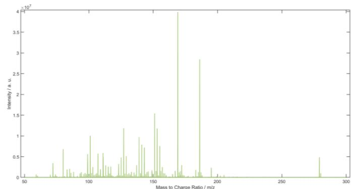
Mass spectrum of a laser desorbed impactor collection with a mean aerodynamic diameter of 95 nm.
