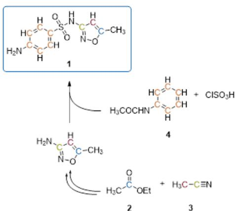
Synthesis scheme for potential position-specific  $^{13}\text{C}$ -labels (colored) or entirely  $^{13}\text{C}$ -labeled sulfamethoxazole (1) using labeled ethyl acetate (2), acetonitrile (3), and acetanilide (4).
