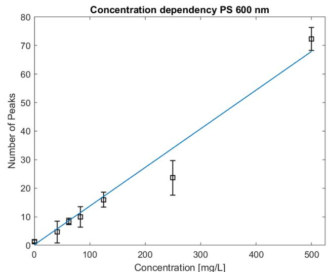
Correlation of the number of detected peaks per measurement with the injected concentration to obtain a calibration curve for 600 nm polystyrene (PS) beads using a linear weighted fit.
