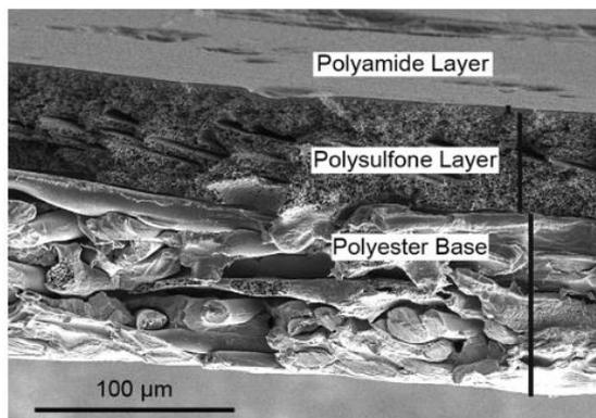
Cross section view of a RO membrane showing the three different layers (1. Polyamide: ~ 100 nm; 2. Polysulfone: ~ 50 µm; 3. Polyester Base: ~ 120–150 µm)<sup>2</sup>
