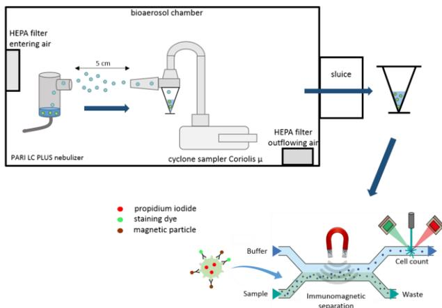
Schematic workflow for experiments with bioaerosols: generation of aerosols with *L. pneumophila* in aerosol chamber with Pari LC Plus Nebulizer, sampling with cyclone sampler (Coriolis  $\mu$ ) and subsequent performing of Immunomagnetic separation (IMS) coupled with flow cytometry (FCM) for quantification of cell concentrations.
