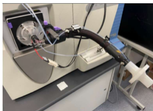
Setup for direct breath measurement via SICRIT-Orbitrap-MS.
