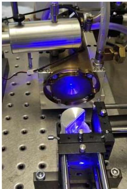
Experimental setup for PAS: resonator cell at controlled temperature and laser diode emitting in the blue range.
