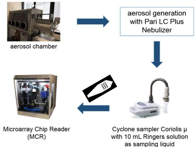
Schematic workflow for experiments with bioaerosols: generation of aerosols with *L. pneumophila* in aerosol chamber with Pari LC Plus Nebulizer, sampling with cyclone sampler (Coriolis  $\mu$ ) and subsequent performing of a chemiluminescence sandwich microarray immunoassay (CL-SMIA) on a Microarray-Chip-Reader Research (MCR-R).
