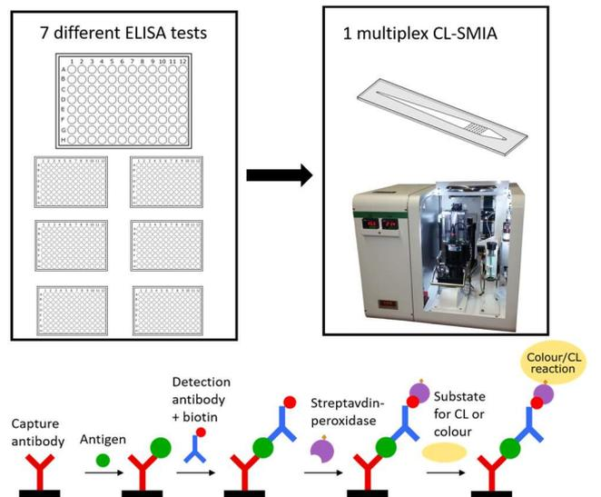
Picture above: Transferring 7 individual ELISA tests to a flow-based multiplex CL-SMIA.
