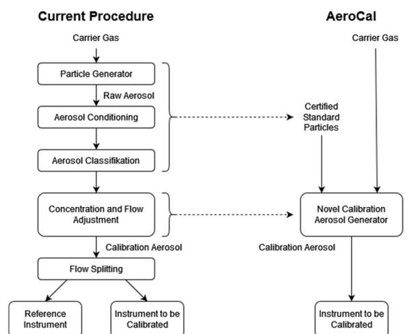
Scheme of the necessary steps in calibration aerosol production for aerosol instrument calibration. Left: Classical calibration. Right: Calibration with the novel calibration aerosol generator developed in this project.
