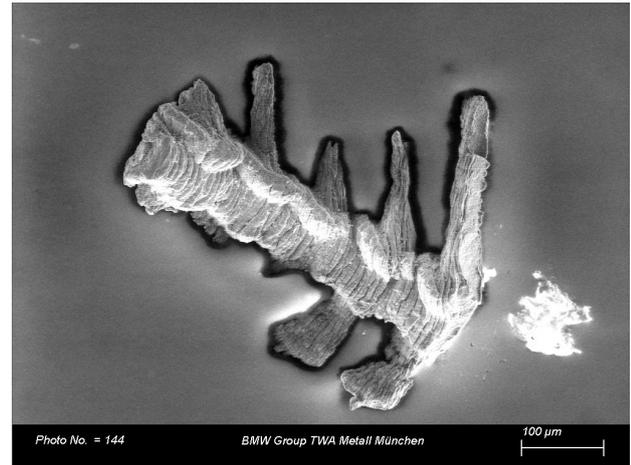
SEM image of a steel particle produced by the hand-held mortar as an example of the highly irregular shapes produced by this method.
