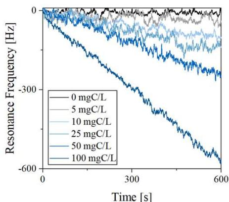
Left side: Scheme of the microfluidic spray-dryer for deposition of NOM solutions onto a QCM sensor chip. Right side: Gravimetric detection of aqueous NOM solutions using the microfluidic spray-dryer. Spray-drying of different concentrated NOM solutions leads to a linear decrease of the measured resonance frequency with time. The slope is dependent on the concentration.
