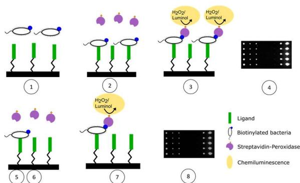
Workflow of the ligand screening: (1) biotinylated bacteria bind on the ligands, (2) Strep-HRP binds on biotin and (3) catalyzes a CL reaction, (4) which is detected by a CCD camera. Then (5) the bound bacteria are eluted, (6) Strep-HRP binds again and (7) another CL reaction is catalyzed and (8) detected.
