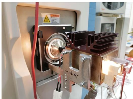
HELIOS-SICRIT-HRMS system during a measurement of an ELPI-collected atmospheric particle sample.
