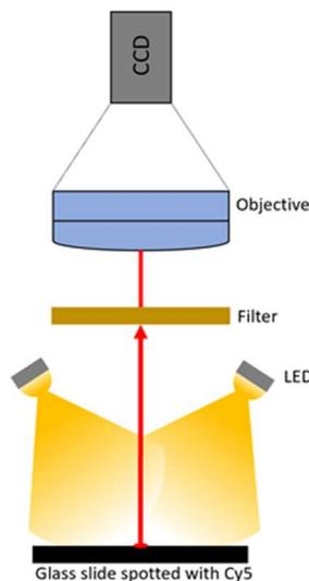
Schematic illustration of the optical read-out unit of the operating device developed within the project DetectRespi. The unit is based on a CCD-camera, an optical bandpass filter (670 nm) and LEDs (Exc.: 645 nm).
