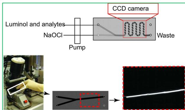
Microfluidic flow-injection aptamer-based chemiluminescence platform.
