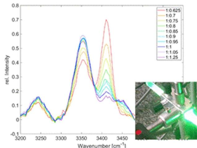
Raman spectra of guanidinium carbonate ( $3414\text{ cm}^{-1}$ ) and nitroguanidine ( $3360\text{ cm}^{-1}$ ) during nitration with different molar ratios ( $Z(\text{G}^+):Z(\text{HNO}_3)$ ). Inset: Raman probe adapter for in-line Raman and Fluorescence spectroscopy
