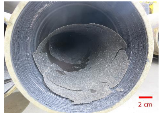
Coarse- crystalline scaling formed in a production pipe with a smooth polymer coating. Due to the poor cohesion, scalings get easily detached and get washed into the filters which eventually leads to blocking of the filters.
