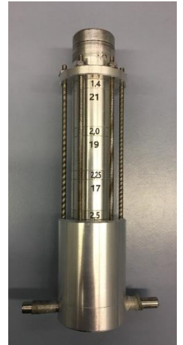
Aerodynamic lens to focus particles in an aerosol flow for a more efficient detection by LIBS.
