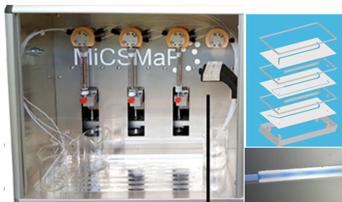
Combined instrument for nanoparticle synthesis with multilayer microreactor
