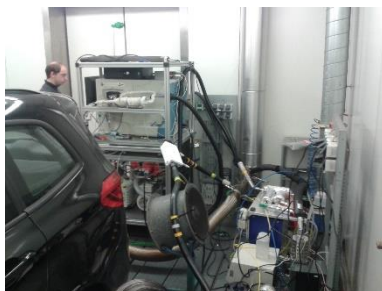
the complete HELIOS/SICRIT/MS on a chassis dyno.
