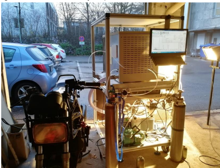
Set up operating in a field campaign: sampling the exhaust gases from an old model motorbike.
