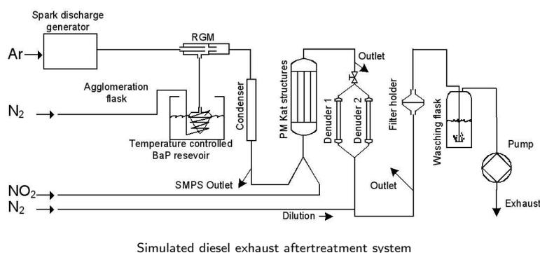
active than PYR towards nitration. In experiments on quartz filters, ca. 75% of coated BaP is converted to 6-nitrobenzo(a)pyrene (6-NBAP) after 3 hours. In our simulated diesel exhaust after treatment system (in the figure) we found the formation of 1- and 6-NBAP. Formation rate was higher at 150°C and decreased at higher temperature.
