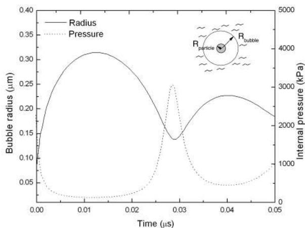
Bubble radius and pressure transients of the water vapor inside the bubbles as calculated from the Rayleigh-Plesset equation. The first maximum in pressure at 29 ns marks the collapse of the bubble; the following modulations are only expected for oscillatory bubble motion
