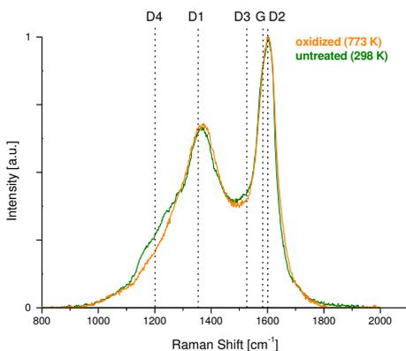
Raman spectra of untreated and oxidized soot
