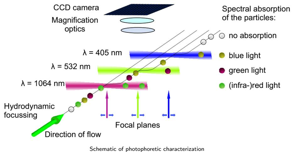
beam are centered in the beam and start migrating in the direction of the beam propagation. An automatic routine for image processing determines the particle velocities.
