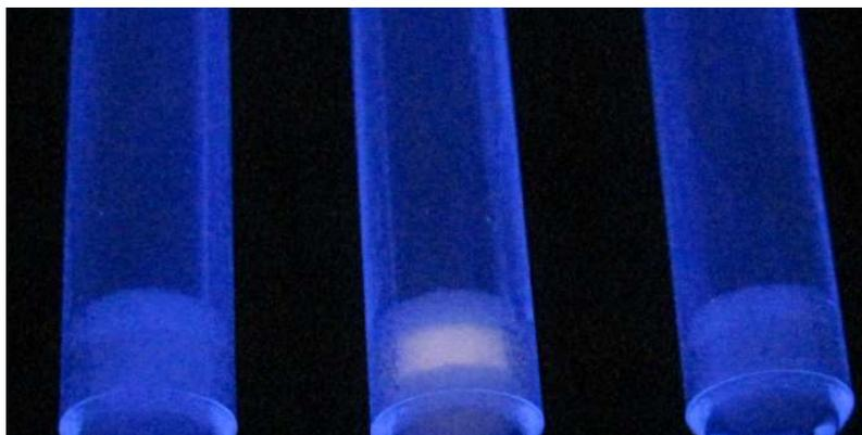
Gel-based immunoassay using quantum dots as label. Left: control (without B[a]P antibody); middle: blank (no B[a]P in sample); right: 5 ng B[a]P in sample.
