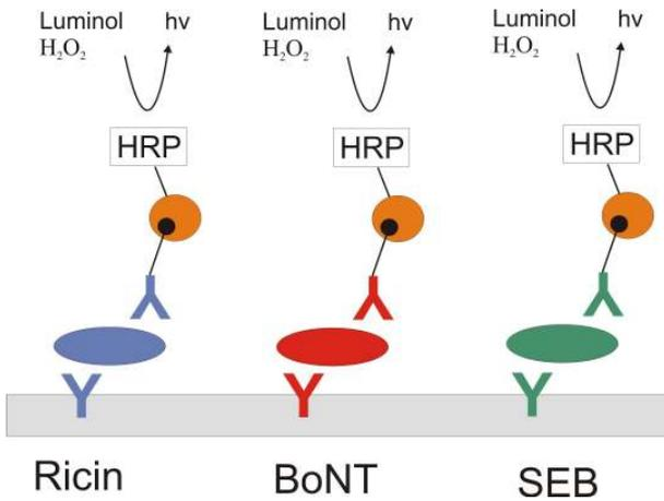
Schematic of the microarray for toxins
