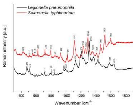
Fingerprint spectrum of *L. pneumophila* (black) and *S. typhimurium* (red). Their amide III band at  $1290\text{ cm}^{-1}$  and  $1310\text{ cm}^{-1}$  respectively, were used for SERS mapping
