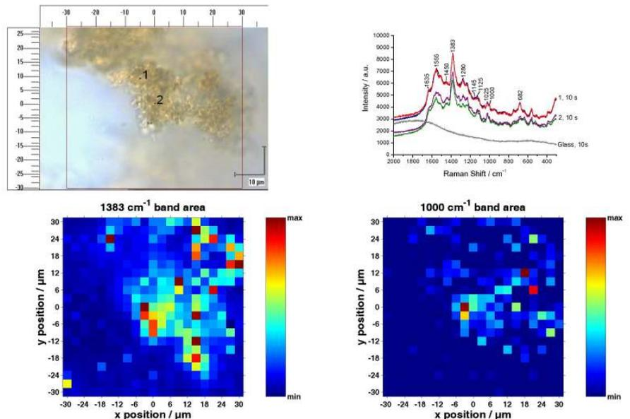
Microscopic image, Raman spectra and spectral mapping of biofilm
