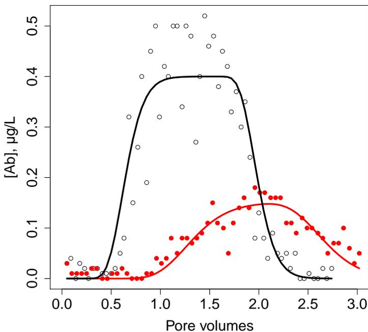
Breakthrough curves of anti-BaP antibodies through silica gel w/ and w/o BaP-coating
