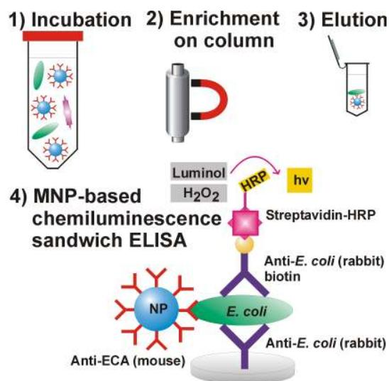
Immunomagnetic separation in combination with CL sandwich immunoassays for the quantification of bacteria
