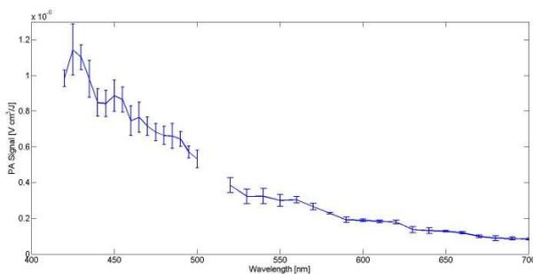
Absorption spectrum of sparc-generated soot, measured with the new instrument
