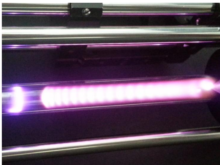
Gas discharge plasma as used for siloxane monitoring
