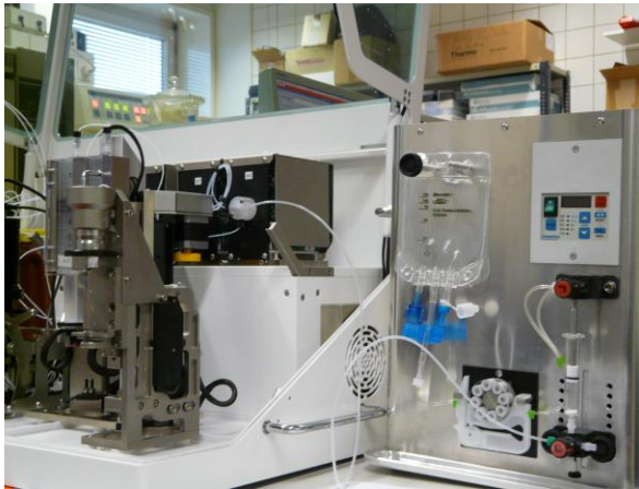
Experimental setup for combined concentration (right) and detection at the MCR 3 (left)
