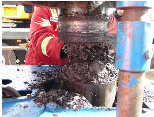
Scalings inside of the stand pipes
