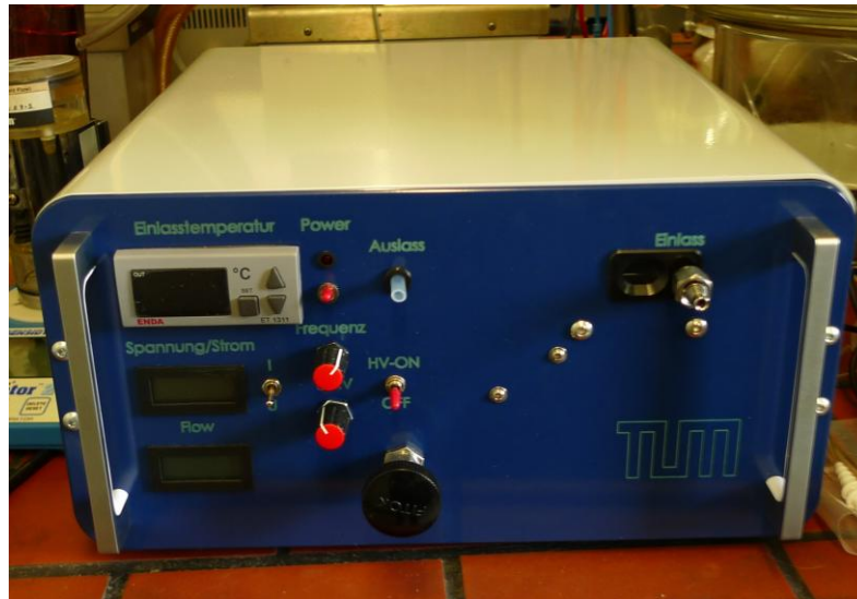
Gas discharge plasma sensor as used for siloxane monitoring
