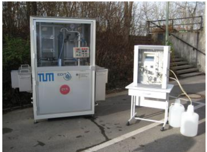
Automated setup for the concentration of 1 m 3 -water samples to a few milliliters by ultrafiltration (left) and monolithic adsorption filtration (right).
