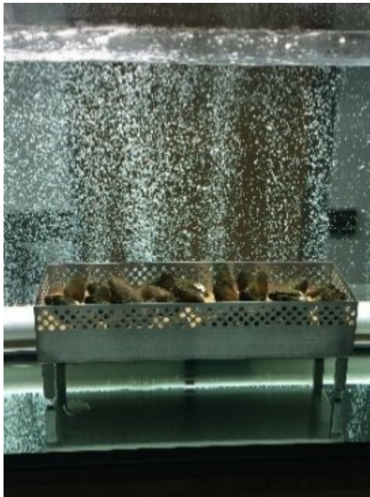
Microplastic exposure of bivalves under standardized laboratory conditions at the Bavarian Environment Agency
