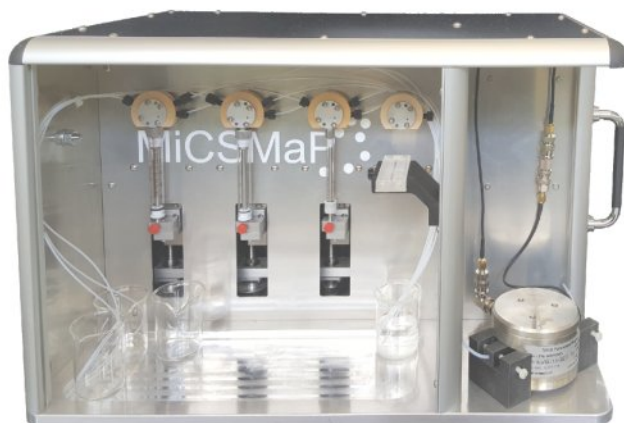
Exploded view of multilayer microreactor with schematic representation of 3D-flow focussing and experimental setup with integrated pumps and T 2 -relaxometer
