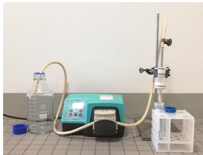
MAF filtration setup used for the concentration of P. aeruginosa from tap water samples.
