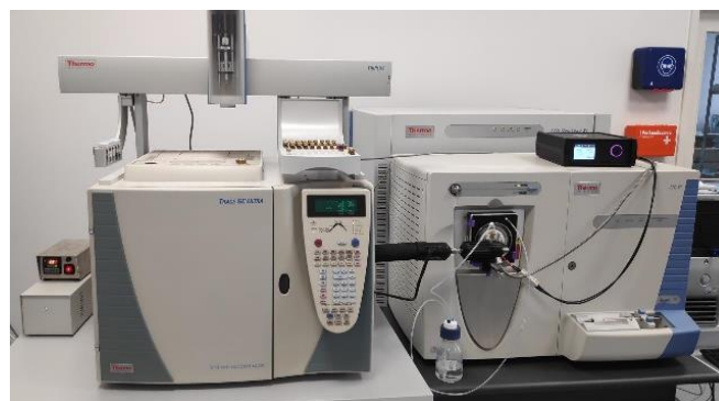
Coupling of GC to a high resolution orbitrap MS via GC-/SPME module and the SICRIT ionization source allowing completely automated measurements.
