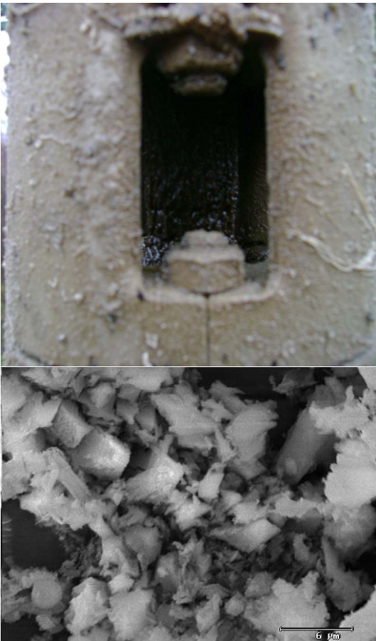
Pump with incrustations and SEM image of the incrustations
