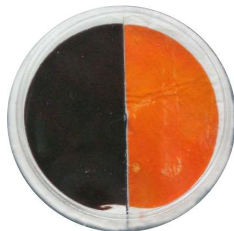
Quartz fiber filter loaded with soot doped with iron compounds (left) and same filter with residues of iron oxides after burning the filter in oxygen stream (right).
