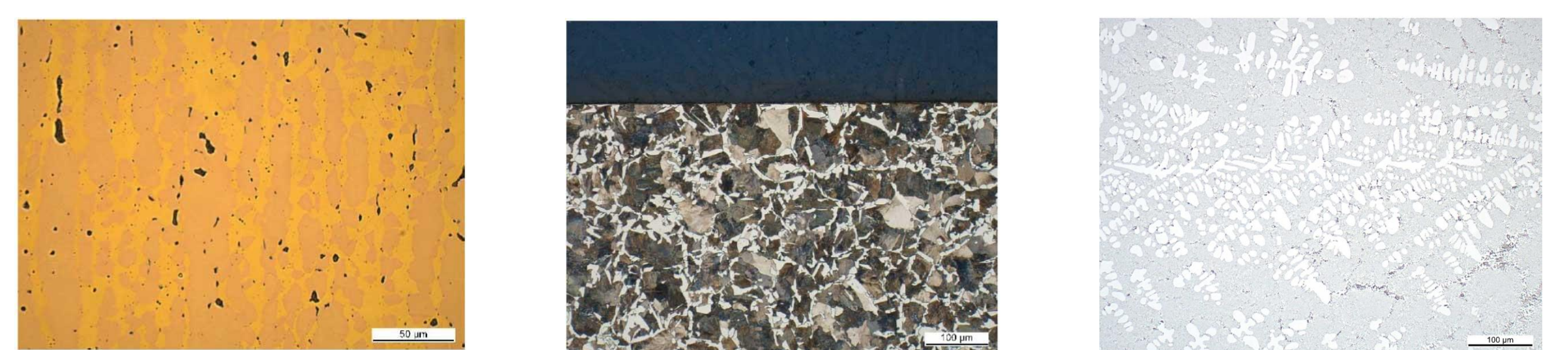
Microstructures of a Cu- (left), Fe- (center) and Al- (right) alloy to visualize present phases and inhomogeneities.
