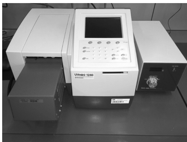
Figure 6.3.1: Spectrophotometer used to study the equilibrium reaction of Rhodamine B.
