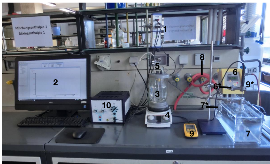
Figure 5.3.1: Experimental set-up with all its parts. (1) Cobra 4 USB-Link, (2) measure software, (3) calorimeter, (4) magnetic stirrer, (5) heating coil with sockets and temperature sensor, (6) thermostat with (6*) buttons to set the temperature, (7) water bath of thermostat with (7*) cooling coil, (8) cooling water valve, (9) digital high-resolution thermometer with (9*) temperature sensor and (10) power supply for the calorimeter.
