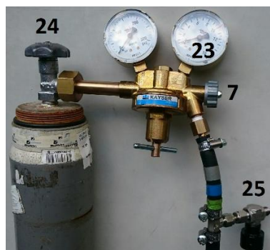
Figure 4.3.4: Pressure reducer on the oxygen cylinder. (7) outlet valve, (23) work manometer, (24) main valve of the oxygen bottle and the venting connection (25).
