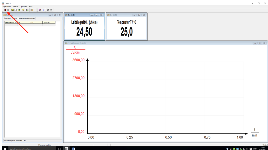
Figure 8.5.2: The arrow points to the red dot that has to be clicked on in order to start a conductivity measurement. When the measurement is running, a black square appears at the position of the red dot. Clicking on it does stop the running experiment.
