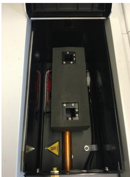
Figure 6.6: The temperature-controlled cell holder.
