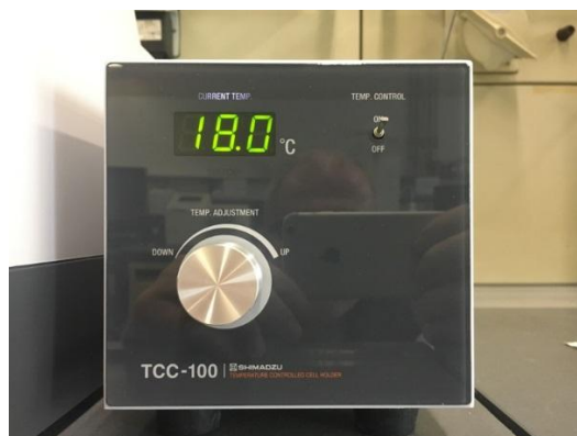
Figure 6.5: Controller for the temperature adjustment of the cell holder.
