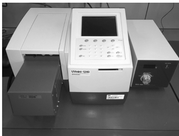
Figure 6.4: Spectrophotometer used to study the equilibrium reaction of Rhodamine B.
