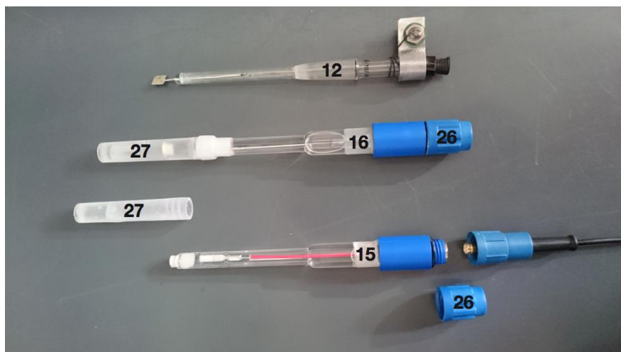
Figure 7.3: Electrodes. (12) Platinum electrode, (15) calomel electrode (with a red wire inside), (16) silver-silver chloride electrode, (26) blue cap, and (27) protective cap.
