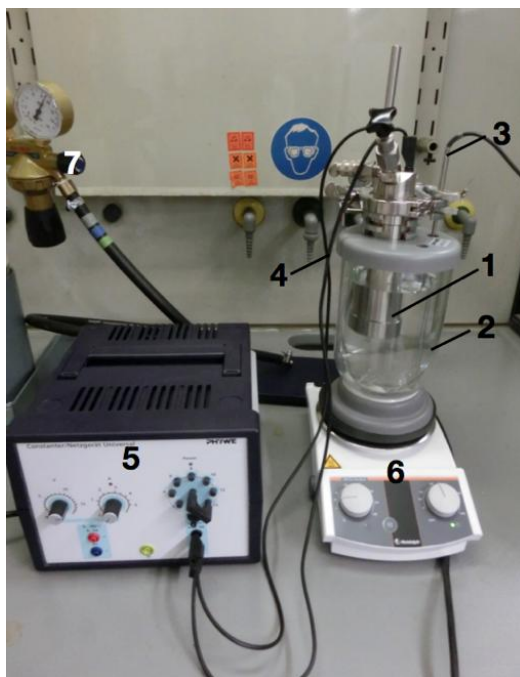
Figure 4.2: Calorimetric setup used for the determination of heat transfer during a chemical reaction; (1) calorimetric bomb, (2) calorimeter vessel, (3) temperature sensor, (4) black connector cords/firing leads, (5) power supply of the ignition unit, (6) magnetic stirrer, and (7) outlet valve.
