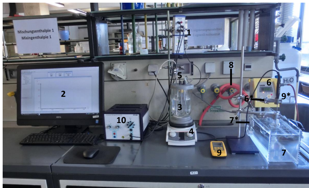
Figure 5.2: Experimental set-up with all its parts. (1) Cobra 4 USB-Link, (2) measure software, (3) calorimeter, (4) magnetic stirrer, (5) heating coil with sockets and temperature sensor, (6) thermostat with (6*) buttons to set the temperature, (7) water bath of thermostat with (7*) cooling coil, (8) cooling water valve, (9) digital high-resolution thermometer with (9*) temperature sensor and (10) power supply for the calorimeter.
