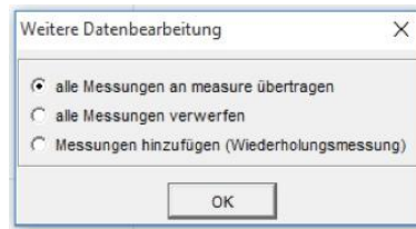
Figure 12.4: Pop-up window that opens when the measurement is stopped. Please select the first option and click OK.
