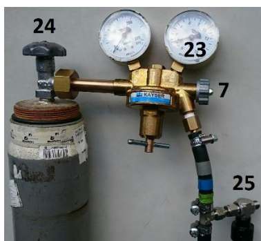
Figure 4.5: Pressure reducer on the oxygen cylinder. (7) outlet valve, (23) work manometer, (24) main valve of the oxygen bottle, and the venting connection (25).
