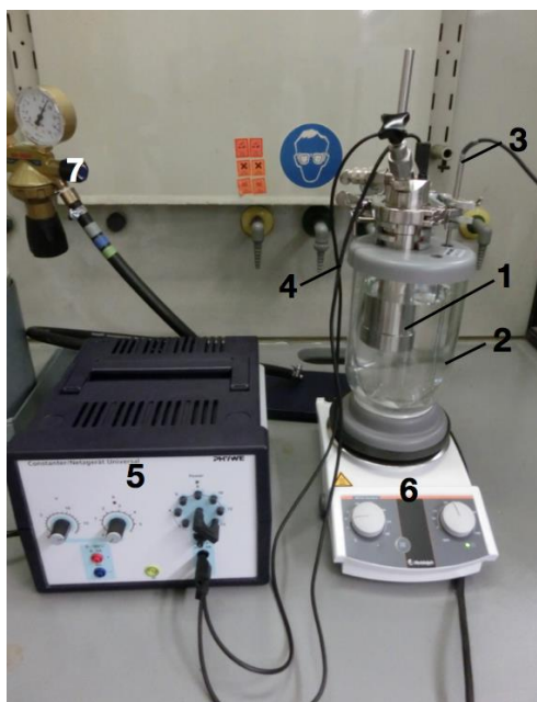
Figure 4.3.1: Calorimetric setup used for the determination of heat transfer during a chemical reaction; (1) calorimetric bomb, (2) calorimeter vessel, (3) temperature sensor, (4) black connector cords/firing leads, (5) power supply of the ignition unit, (6) magnetic stirrer and (7) outlet valve.
