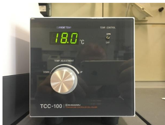
Figure 6.3.2: Controller for the temperature adjustment of the cell holder.
