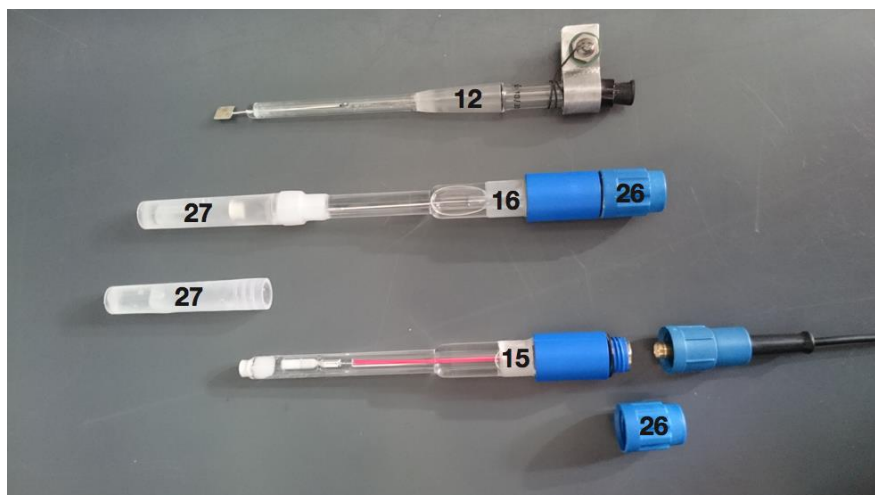
Figure 7.3.3: Electrodes. (12) Platinum electrode, (15) calomel electrode (with a red wire inside), (16) silver-silver chloride electrode, (26) blue cap and (27) protective cap.
